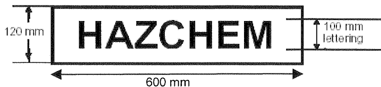
Figure 13.1 Form and dimensions of outer warning placard
